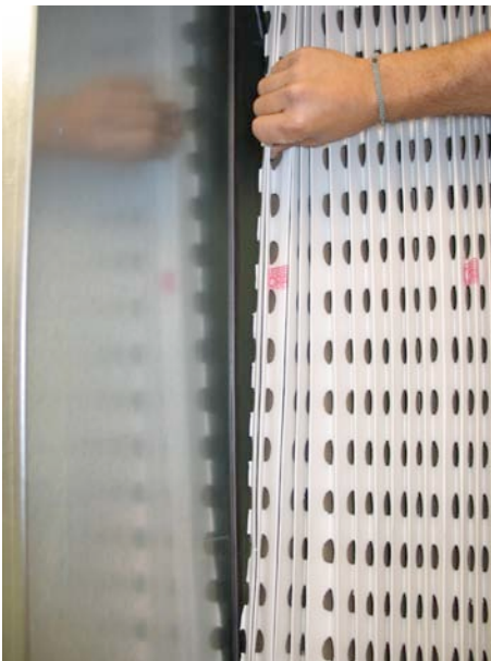
Lay the folded filtering paper on the filter carrying guide and bring the metal band to the end so it covers the magnetic profile.
